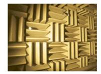
72 frequency response measurements are taken at different points around the loudspeaker, in one of four anechoic chambers. This allows for accurate analysis of a speaker's total performance before the listening tests even begin.
